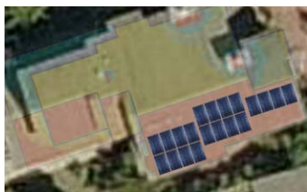
Figure 6: Outline of the building, color coded solar potential and module placement on the roof.
