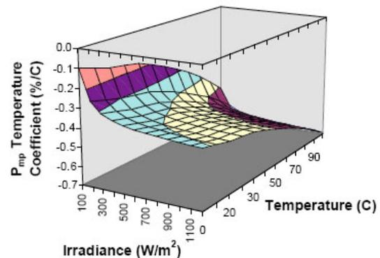
Fig.1: Temperature coefficient for  $P_{mp}$  for an ASE Americas ASE-300-DG/50 module as a function of irradiance and cell temperature.[2]
