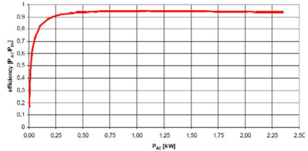
Figure 3. Efficiency curve for the Sunny Boy 2500U (courtesy of SMA-America).
