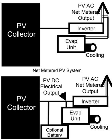
Figure 1. Net Metered PV, AC & DC HVAC.
