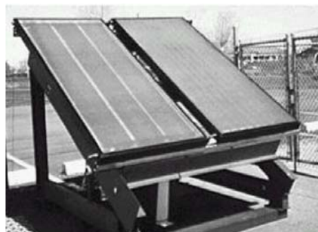
Figure 3 Phototherm PV/T on Left, SunEarth Empire thermal collector on right. (Photo courtesy of NREL and Solar Design Associates)
