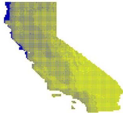
Fig. 4: Flat Plate map for places with greater than 4.930 kWh / day average, or 1,800 kWh / kW installed capacity per year.
