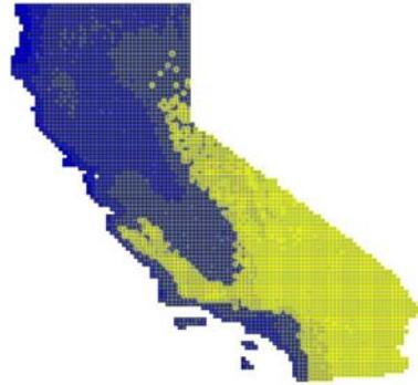
Fig. 3: Flat Plate map for places with greater than 6 kWh / day average, or 2,190 kWh / kW installed capacity per year.
